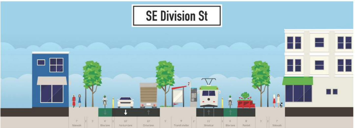
DIVISION STREET AND BUILDING IMPROVEMENTS : Potential cross-section of improvements for SE Division St. includes future high capacity transit, bike and pedestrian infrastructure. Storefront improvements and business investment along corridor should be appropriately scaled to the surrounding neighborhood.
